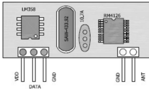
The DL-RXR4126 module has 5 pins, which are defined in the following table:
