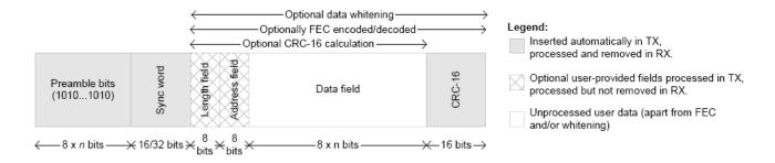
In addition, CC2500 supports the transmission mode of fixed packet length, variable packet length and unlimited packet length. Different packet lengths have different configuration and control modes. For details, please refer to CC2500 chip specification.
