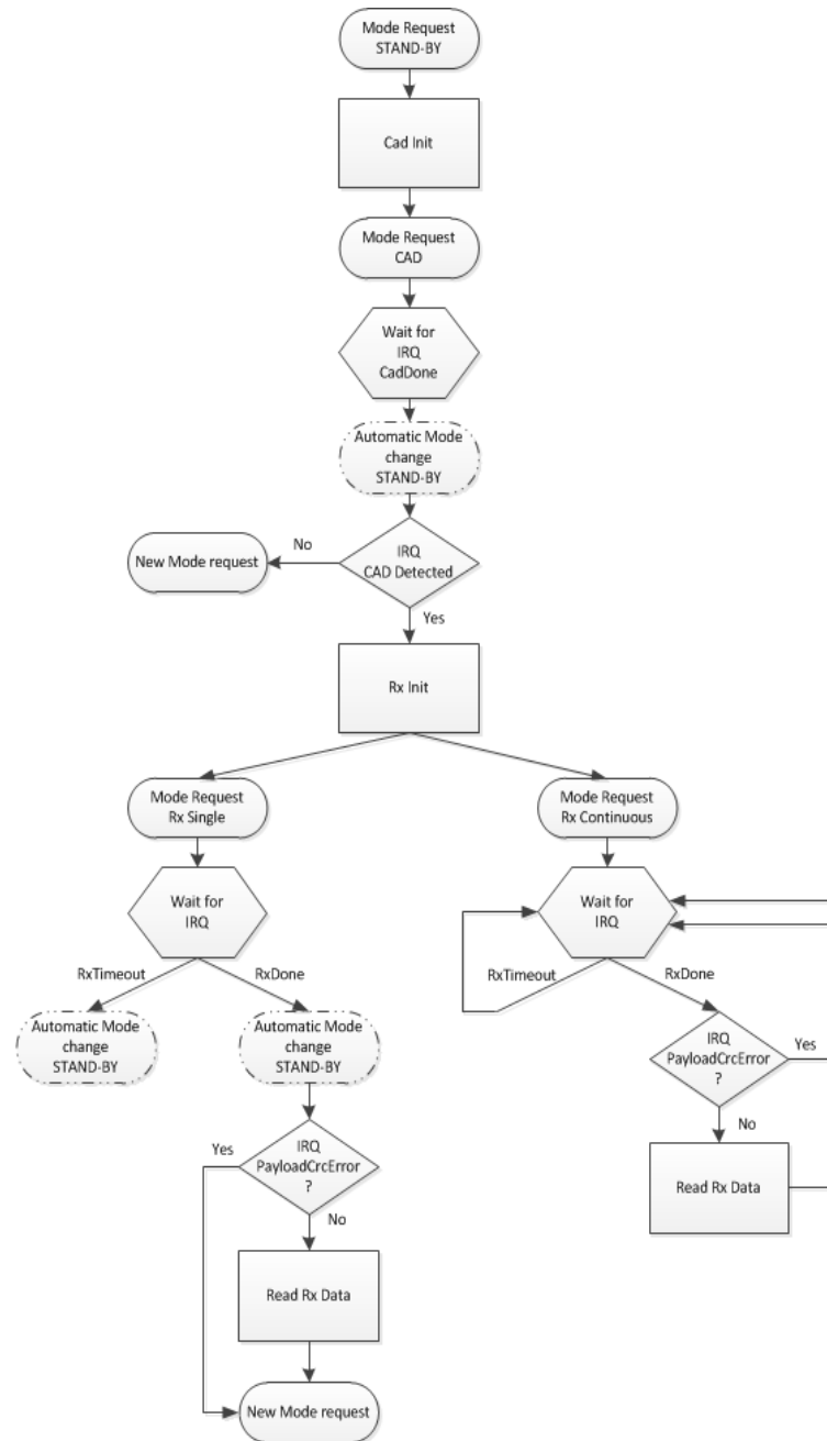
Figure 10. LoRa™ CAD flow
