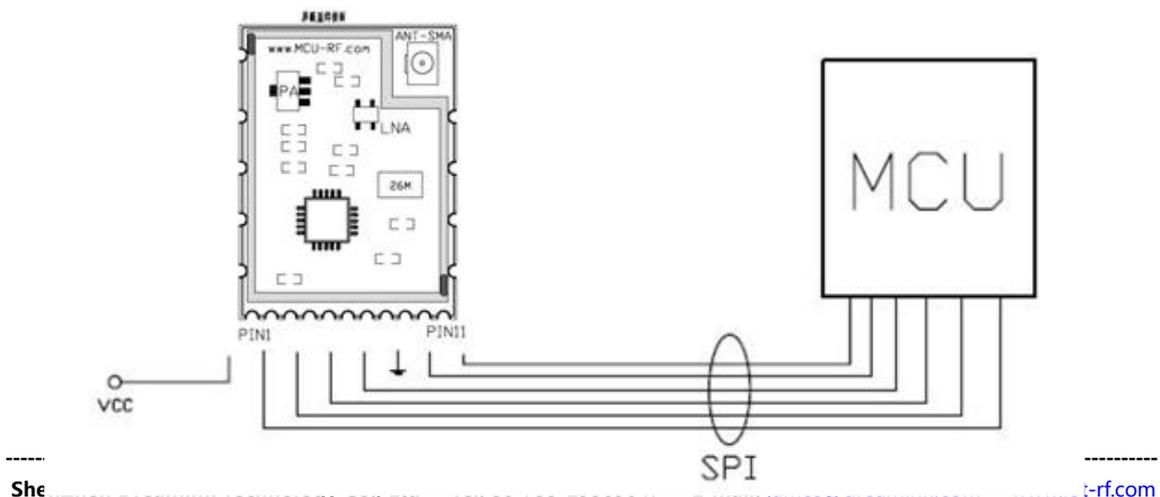
Figure 2: Wiring diagram for module application
