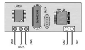
The DL-RXR4126 module has 5 pins, which are defined in the following table:
