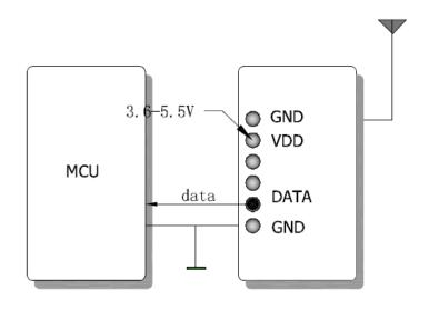
Figure 2: Wiring diagram for module application
