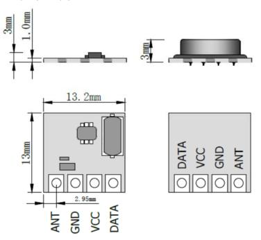
The DL-TX19 module has 4 pins, which are defined in the following table
