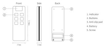
Indicator: blue light as default Buttons: 6 keys Supporting RF Module: 6-channel switch control receiving module
